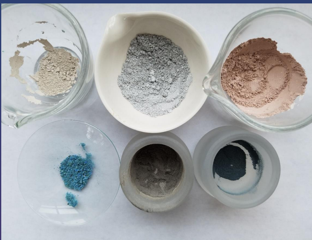
Figure 1. The pigments preheated (top row) and after heating (bottom row). From left to right: Sample A, Sample B, Sample C
