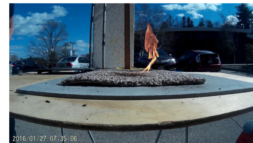
Picture 3: 1 mL of lighter fluid on Dark Carpet, producing a flame height of 23.265 cm
