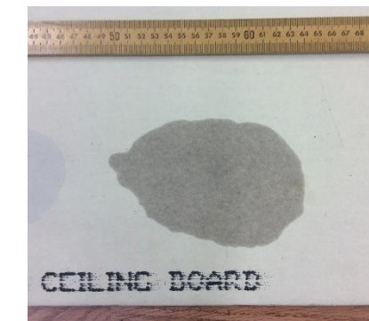
Picture 2: 4mL pool size on Drywall, with an average area of 100.5858 cm 2 .
