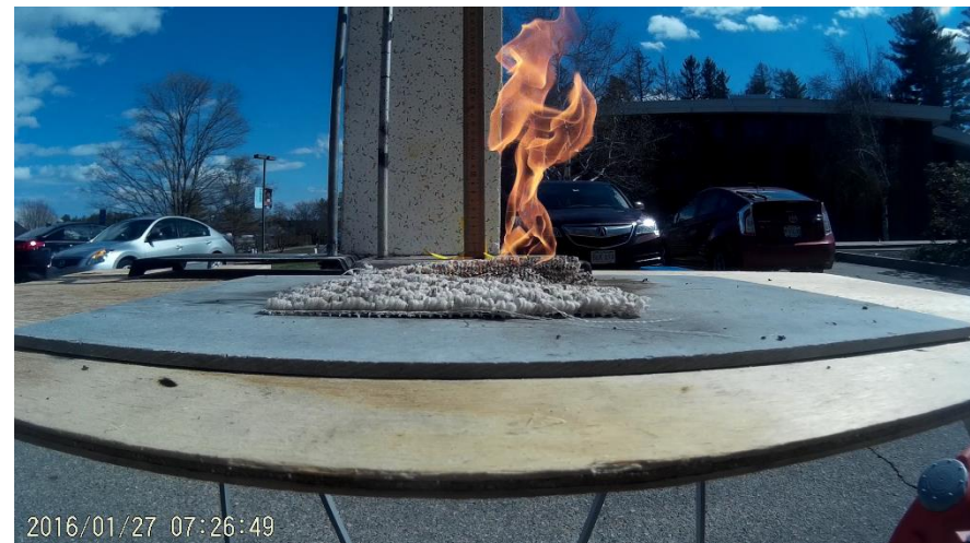
Picture 1: 2mL of lighter fluid on light carpet, producing a flame height of 32.464 cm.
